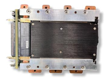
REN VPX FlatPAK is a single slot VPX card carrier, it can be supplied for 3U and 6U VPX cards and can be used on its own or in clusters. It uses 1-slot VPX backplanes in the SOSA format along with VITA 62 PSU backplanes to provide a modular way of utilising VPX cards.
