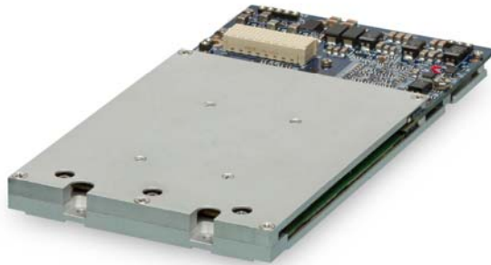
StorePak Air Cooled SX6S-XMC (with XMC "stack" connector)
